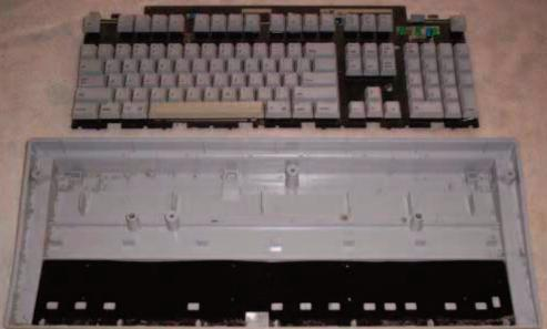
looking at the mat sitting in the back part of the casing. A brush, a can of air, and even some type of cleaner will help get it looking brand new. You can also take the main part of the keyboard out completely so you can wash both the top and bottom plastic casing. Just be sure to watch the ADB ports on both sides toward the top – they are easy to get out and back in, but use caution.
